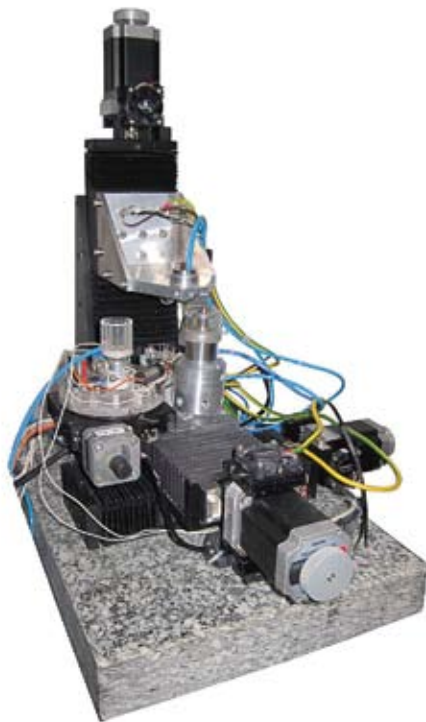
Figure 4. A machine developed by FBK for making micro-grinding tools. It combines three processes: grinding, coating and EDM.
