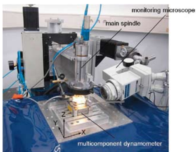
Figure 2. A precision grinding and milling machine applying the tools of Figure 1. Working area 100 \times 100 \times 100 \text{ mm}^3 , positioning resolution < 0.1 \text{ }\mu\text{m} .
