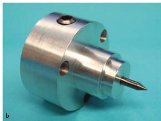
Figure 3. A monolithic hydraulic expansion device for clamping a tungsten carbide shank that is to be ground into a micro end mill. The device symmetrically compresses the shank to realise a rotational accuracy better than 0.2 \text{ }\mu\text{m} .
