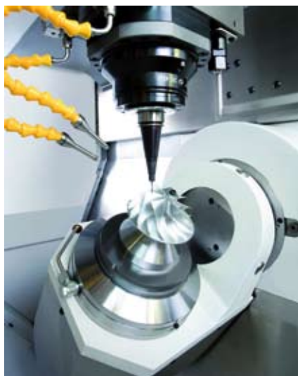
Figure 1. High-speed precision milling of an impeller with a GF AgieCharmilles Mikron HSM 400 LP machining centre.
