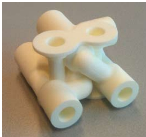
Figure 4. A manifold, produced in one piece, using the limited space optimally, yet showing smooth corners.
