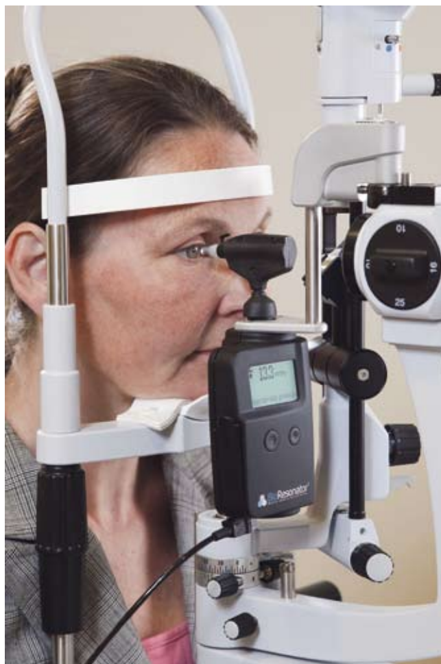
Figure 10. A PiezoWave motor used for measuring the pressure in the vitreous body of an eye.
