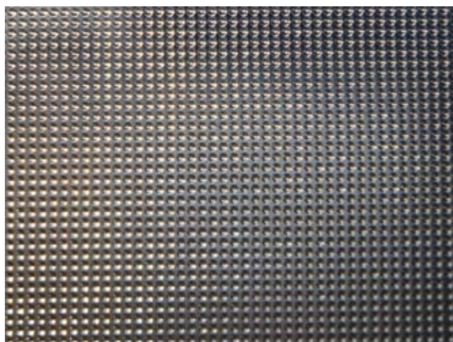
Figure 6. An optical structure printed on foil.
