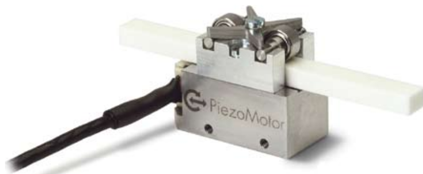
Figure 1. A Faulhaber PiezoMotor PiezoLegs 6N linear motor. The piezo elements are enclosed in steel. Above two ball bearings for guiding the ceramic driving rod. Holding force 7 N, resolution < 1 nm, maximum speed 20 mm/s.
