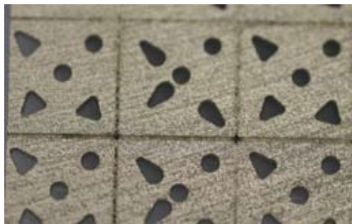
Figure 7. High-aspect-ratio periodic structure for use as a microreplication mould.
