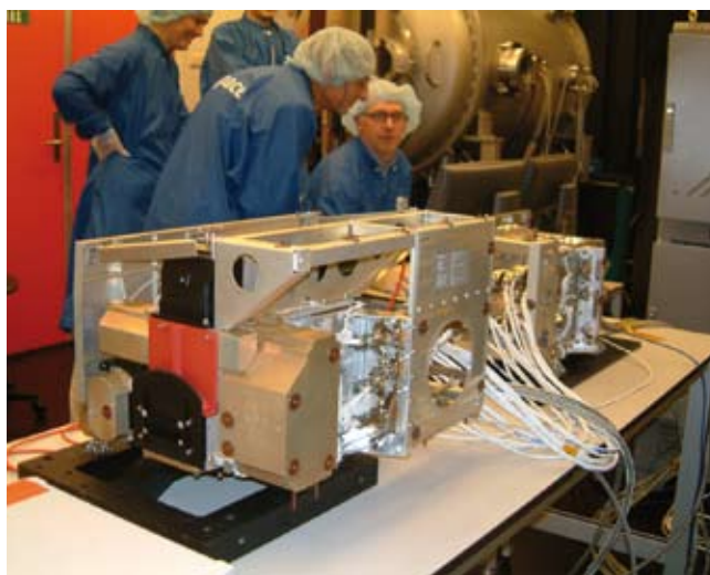
The Ozone Monitoring Instrument (OMI) before shipment. OMI, built by a consortium in Zuid-Holland, measures ozone and other pollutants in earth's atmosphere from space. It is the first instrument ever for globally monitoring atmospheric ozone concentrations on a daily basis.
