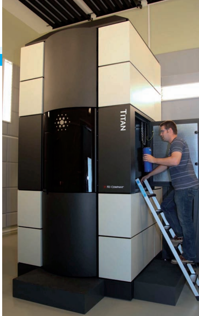
Figure 5. The Titan Krios, a TEM operating with 300 kV, for studying frozen-hydrated biological samples.
