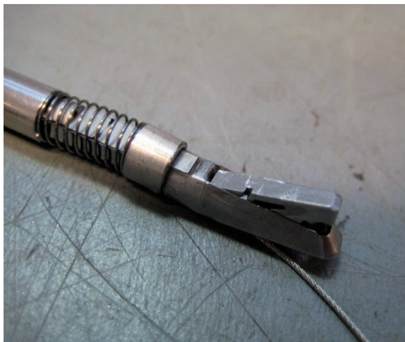
Figure 6. The prototype fitted with an end effector from a standard punch for presentation purposes. This end effector is activated using a steel wire connected to the jaw of the punch.
