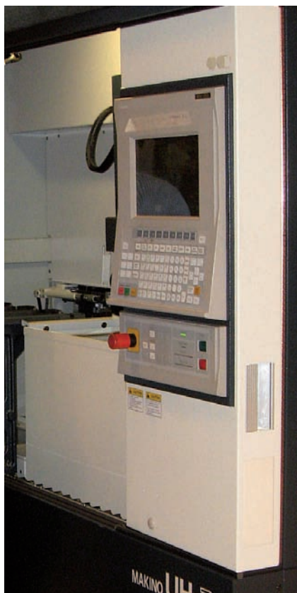
Figure 4. A Makino UH2 advanced wire spark erosion machine for ultrathin wire, 0.03-0.2 mm.
