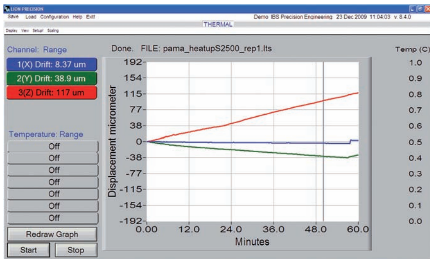
Figure 2. The drift in an uncompensated machine after an hour of warming up at a speed of 2,500 rpm.
