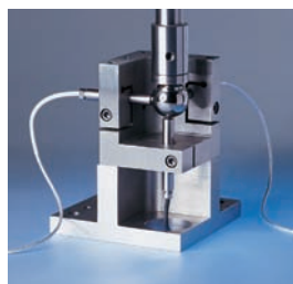
Figure 1. A Masterball is attached to the spindle. The probe nest, mounted firmly to the machine's table, is equipped with sensors. The capacitance sensors measure the (change in) distance to the Masterball.
