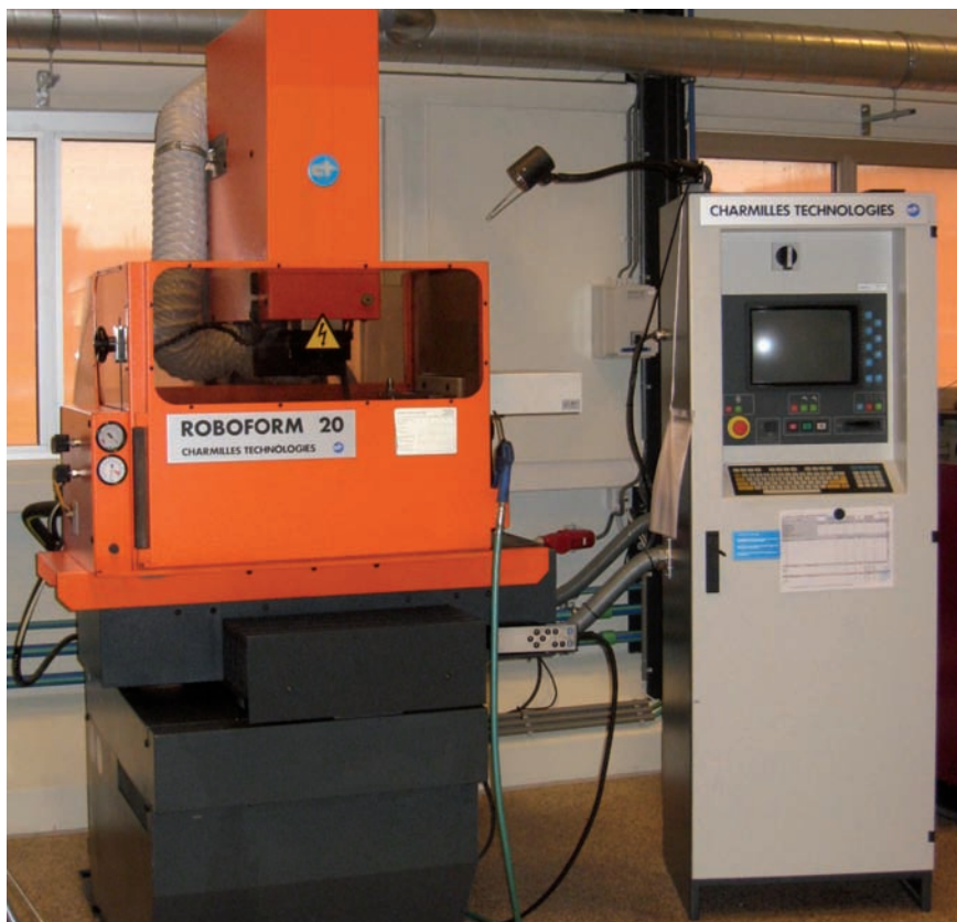
Figure 5. A Roboform die sinking spark erosion machine with control cabinet on the right.
