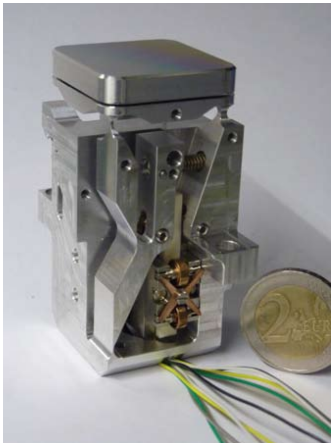
Figure 4. Monolithic tip/tilt mirror.
