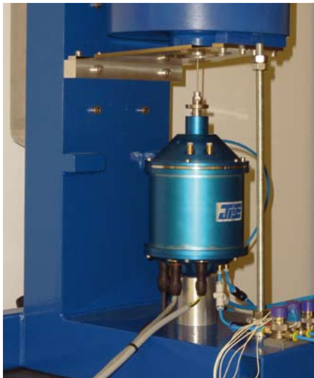
Figure 5. HiPack 'soft' actuator for telescope mirrors.
