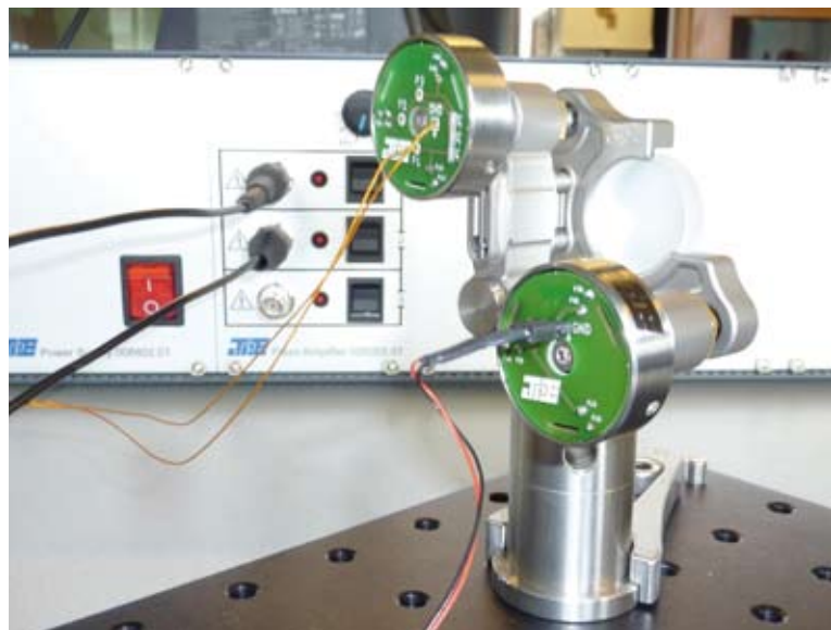
Figure 7. PiezoKnob, motor and dedicated electronics for cryogenic environments.
