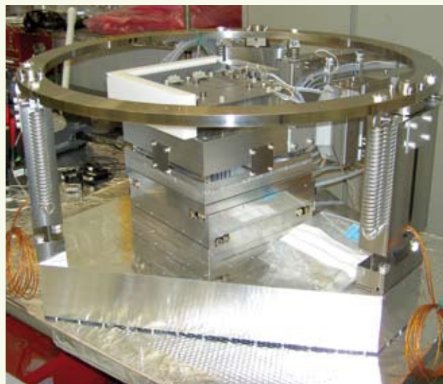
The high-precision stage in IMS's eMET proof-of-concept system as delivered by Philips Innovation Services.
