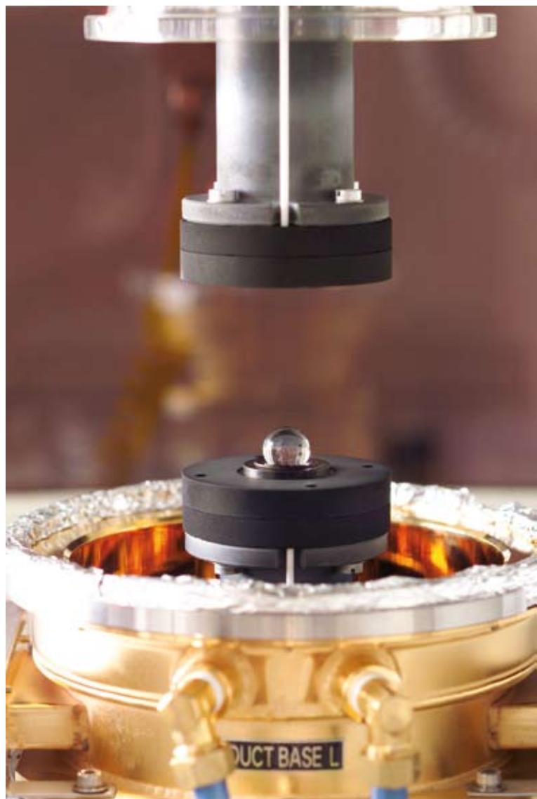
Figure 7. The Precision4 \mu process for glass moulding.
