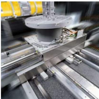
High precision and equal course: detail of a manipulator for an X-ray measuring machine.
