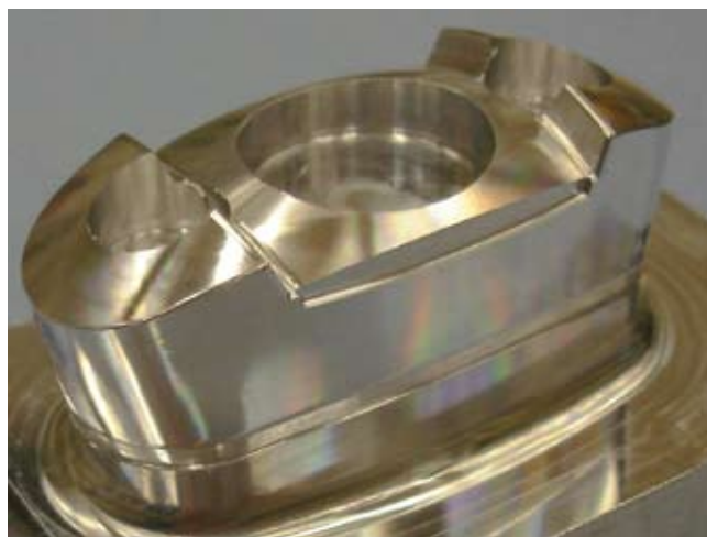
Figure 9. A simultaneously 5-axis milled product with excellent surface quality.
