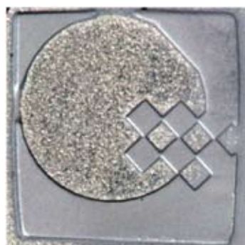
combination of standard lithography and ECM leads to microstructures in mould inserts for replication in tool steels, see Figure 4.
