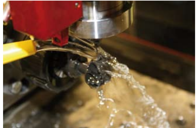
Figure 2. Micro-EDM milling of a turbine impeller ( \varnothing 20 \text{ mm} ) made from \text{Si}_3\text{N}_4\text{-TiN} . (Photo courtesy K.U.Leuven)
