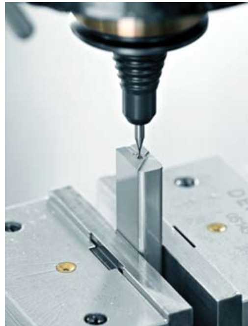
Figure 5. HSM milling a precision part.
