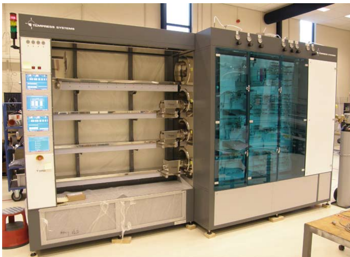
Figure 4. Tempress equipment developed within the Memphis project: the LPCVD and atmospheric oxidation furnace. From left to right: touchscreens for process control; loader units (the upper one for the newly developed ATM process, the lower three for LPCVD); and four gas systems, one for each process (behind them, not visible, the process chambers).
