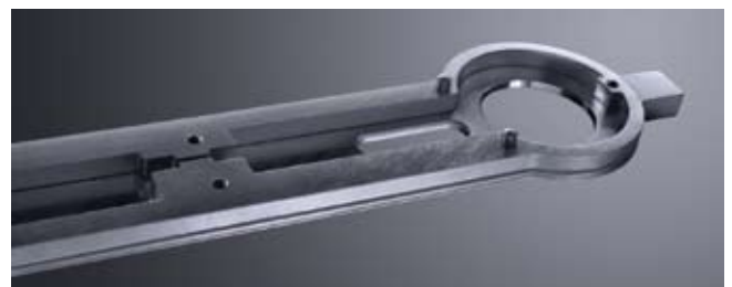
Figure 2. An example of a laser cut and welded product from sheet steel that replaces a much more expensive piece milled from solid.
