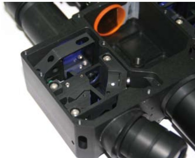
Figure 4. Detail of the prototype, showing the adjustment of the lenses using elastic hinges.
