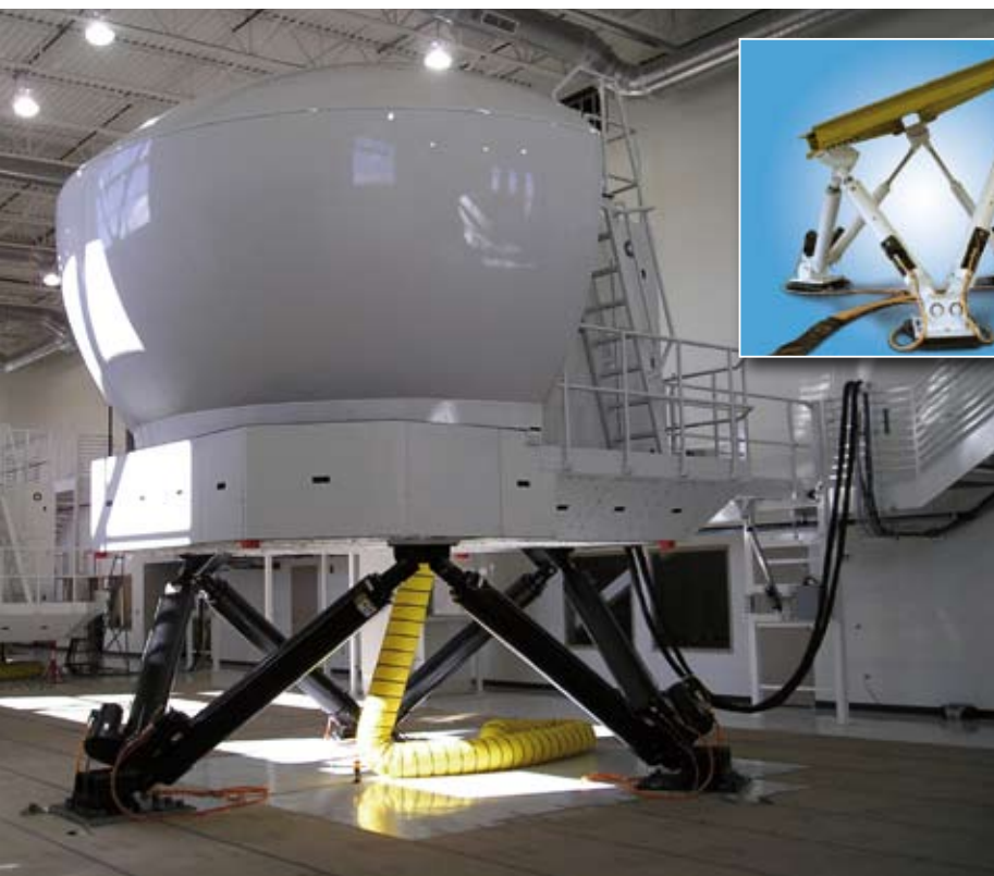
Figure 1. Bosch Rexroth Systems and Engineering developed and realized the motion platform (inset) for a flight simulator.
