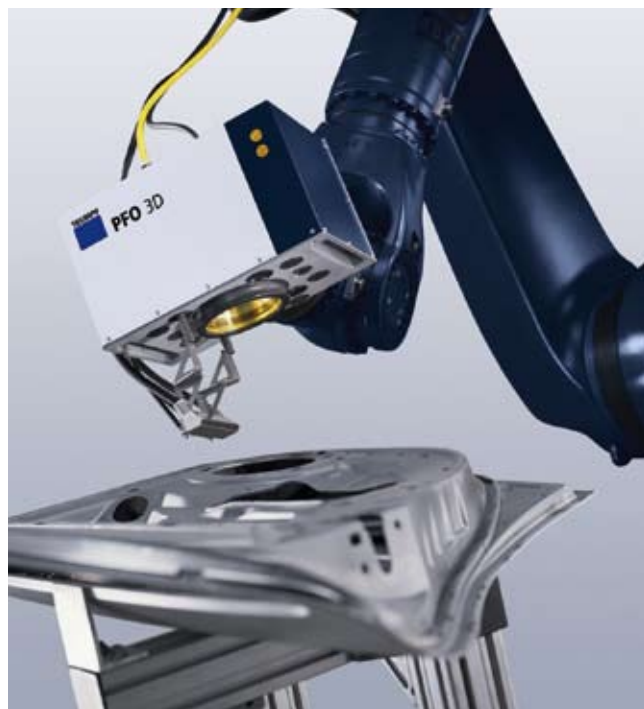
Figure 7. A remote laser system with a PFO 3D (PFO: Programmable Focusing Optics) mounted on a robot for welding a car door. After rough positioning by the robot the PFO focuses the laser spot accurately.
