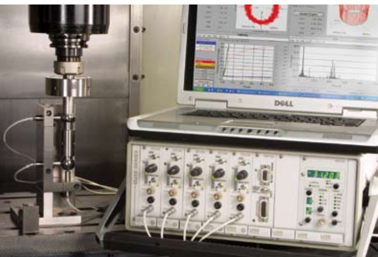
Figure 4. Double-ball set-up for IBS's Spindle Error Analyser.
