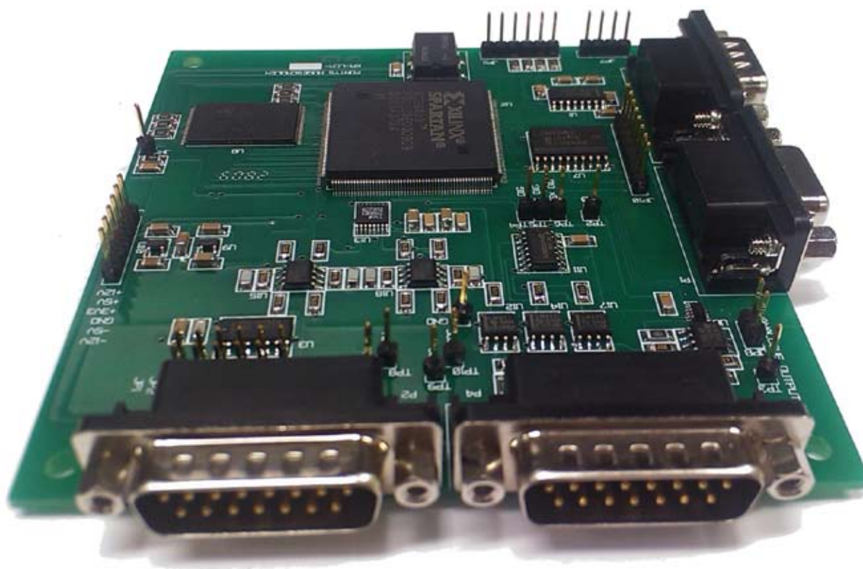
Figure 5. The final result: a high-end, low-cost motion control board.
