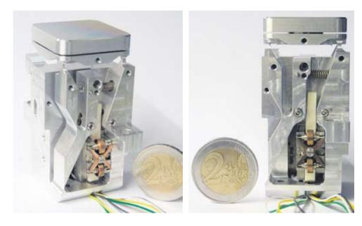
angular tip/tilt resolution of 1.22  $\mu$ rad equals a displacement resolution of the actuator bar of 1.51  $\mu$ m. And the specified angular tip/tilt range of +/- 5.24 mrad equals a displacement resolution of the actuator bar of +/- 6.47 mm. These are feasible requirements for the actuator.
