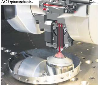
Composite picture of the NANOMEFOS sensor measuring a freeform and a CAD drawing of the sensor design. (Photo: L. Ploeg; editing: L. Cacace)
