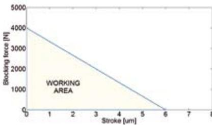
Figure 3. Working area of a piezo actuator.
