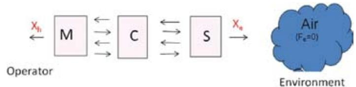
$h_{22}(s) = X_e/F_e$ , output admittance at slave with fixed master:
