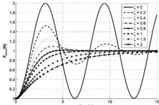
Figure 7. Step response for different values of  $\zeta$  of the model.
