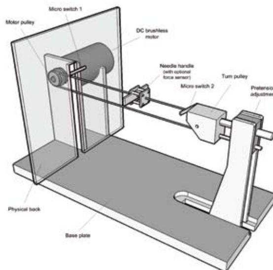
Figure 3. The epidural needle insertion simulator design.
