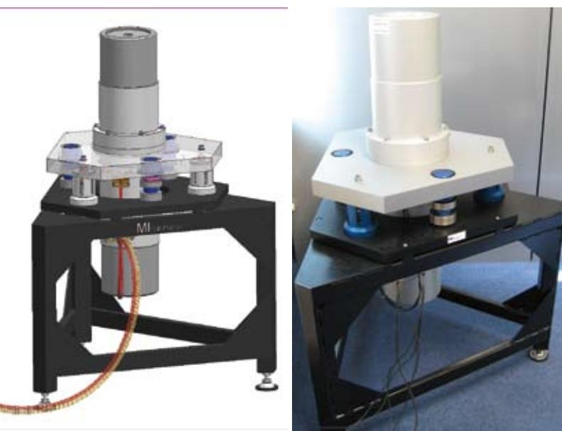
Figure 9. Vibration isolation platform (drawing on the left, actual construction on the right) with three velocity sensors.
