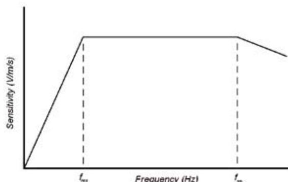
Figure 4. Response curve of a geophone.
