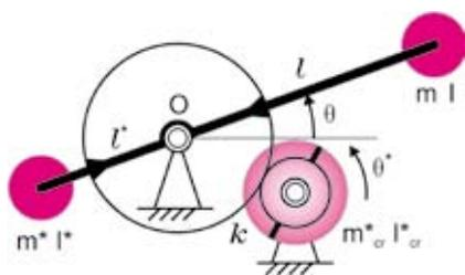
Figure 1. Balancing principle with a Separate Counter-Rotation (SCR).
