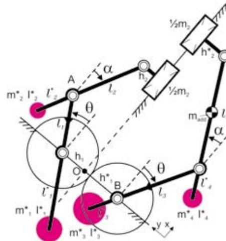
Figure 10. Balanced crank-slider by specifically designed counter-mechanism.
