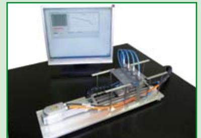
Set-up for thickness measurement using the pneumatic metrology.
