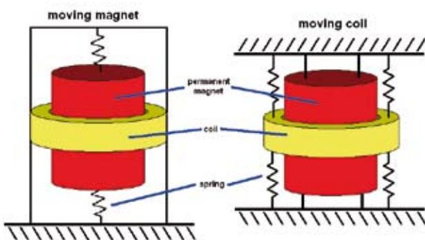
Figure 3. Geophone topologies: moving magnet (left) and moving coil.
