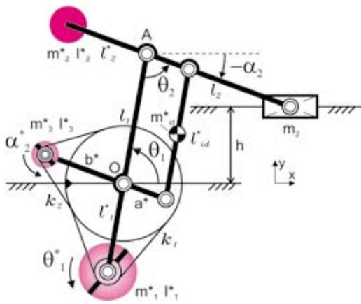
Figure 8. CRCM-balanced crank-slider mechanism deduced from Figure 7.
