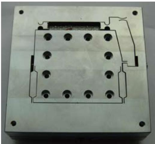
Stroke = 50-250  $\mu\text{m}$ ;  $C = \sim 5 \cdot 10^6 \text{ N/m}$ ;  $F_{\text{res}} = \sim 1 \text{ kHz}$ ; UHV compatible
