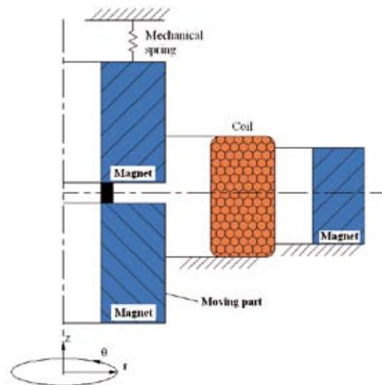
Figure 6. Geophone with passive magnetic spring.
