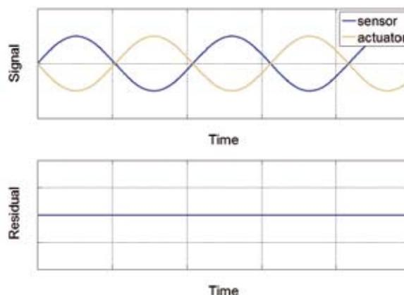
Figure 15. Active damping of (submicron) vibrations by piezo components.
