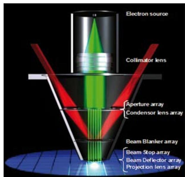
Figure 2. Schematic of MAPPER's massively parallel e-beam column.
