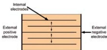
Figure 4. A multi-layer piezo component.
