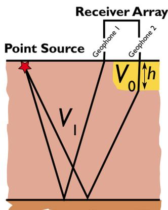
Figure 1. The principle of seismic measurement.
