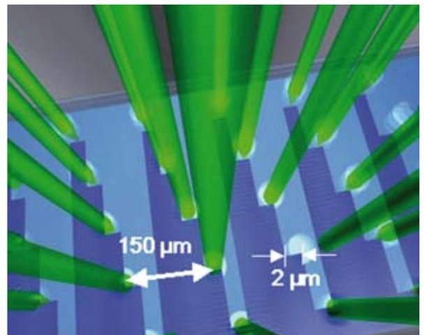
(b) Zoom of (top view of) beam positions in Electron Optics (EO) slit.
