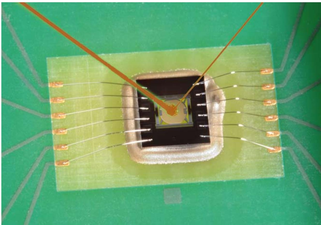
Figure 2. A micro-mirror fabricated using MEMS technology.
