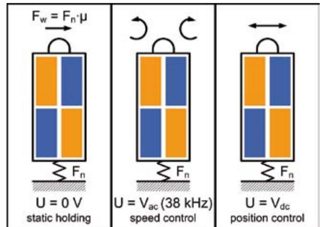
Figure 12. Three functions incorporated in one piezo motor element.
