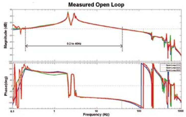
Figure 10. Measured open-loop system transfer functions with three sensors.
