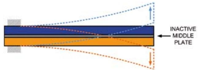
Figure 5. Bending mode of a piezo actuator.
