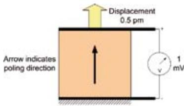
Figure 2. Piezo technology enables subnanometer positioning.
