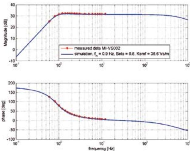
Figure 8. Frequency response of the sensor.
