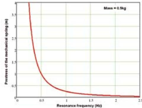
Figure 5. Preload of the spring with constant mass as function of  $f_{res}$ .
