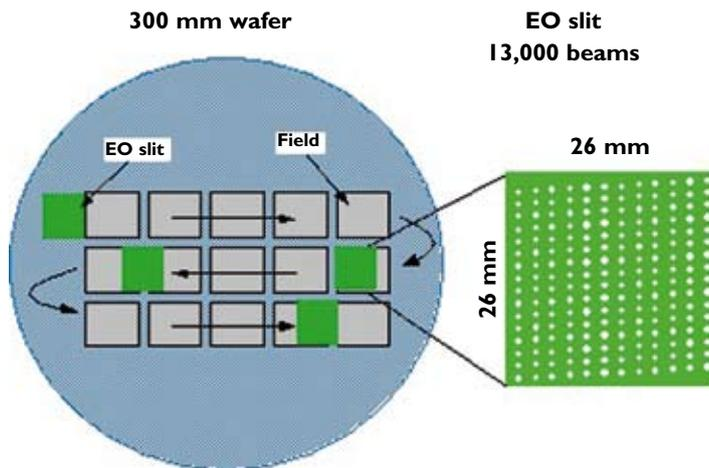
Figure 1. MAPPER's massively parallel electron beam approach. (a) Arrangement of electron beams and writing strategy.
