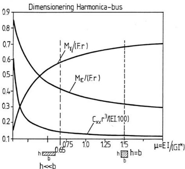
Figure 2. Dimensioning graphs for a harmonica bush, [1].
