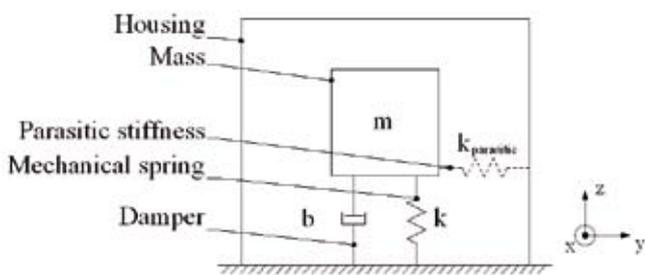
Figure 2. Mechanical geophone representation.
