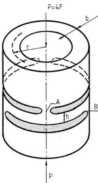
Figure 1. The harmonica bush design principle [1].
