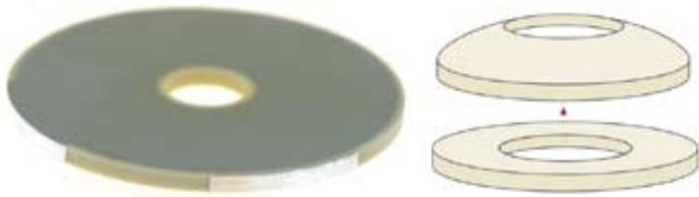
Figure 7. A ring bender and its principle of operation.
