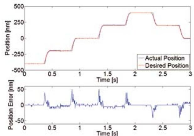
Figure 13. Position profile steps of  $200 \text{ nm}$  by a stage using Nanomotion piezo motor technology.
