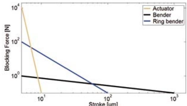
Figure 6. Comparison of blocking force vs stroke for piezo actuator, bender and ring bender.
