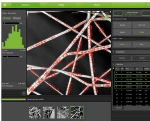
A screen shot showing an example of the Fibermetric system's automated measurements of fiber diameters.
