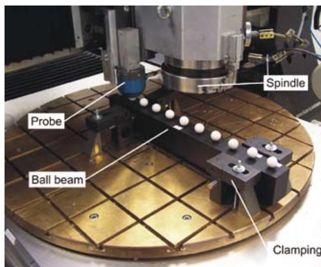
Figure 4. MT-Check installed on a machine tool.
