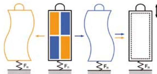
Figure 10. Principle of the dual mode standing wave.
