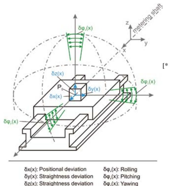
Figure 1. Geometrical deviations of a translational axis [1].
