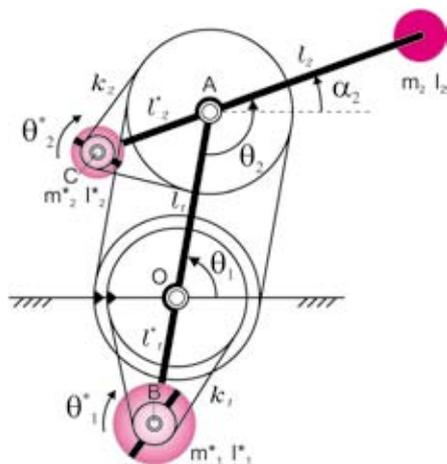
Figure 5. CRCM-balanced double pendulum with low inertia.
