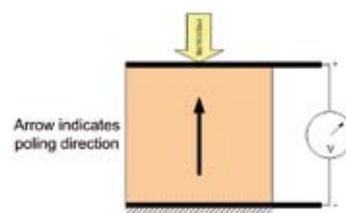
Figure 1. In response to pressure piezo material generates an electrical field.
