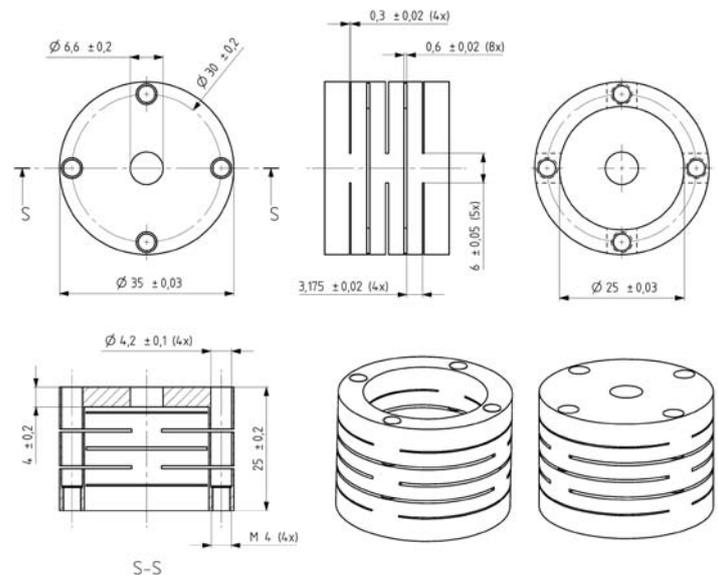
Figure 3. A final design of the harmonica bush.
