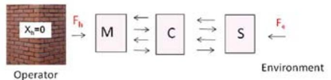
$h_{21}(s) = X_e/X_h$ , position tracking in free motion:
