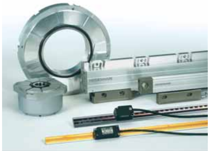
Figure 6. A selection of linear and angular position encoders for direct drives. Signal periods are as low as 4 \mu\text{m} or 36.000 per revolution. Maximum interpolation errors are as low as \pm 0.04 \mu\text{m} or \pm 0.4'' .
