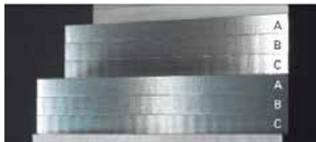
Figure 3. Quality of the milled workpiece surface for: A: Position encoder with \pm 0.4 \mu\text{m} interpolation error. B, C: Position encoder with \pm 1 \mu\text{m} interpolation error.
