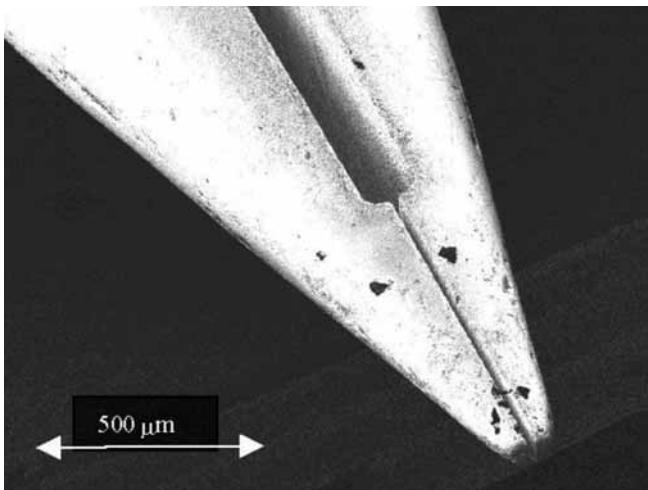
Figure 6.5. SEM micrograph of a micro reservoir pin with a capillary slot 15  $\mu\text{m}$  wide by 600  $\mu\text{m}$  long and a reservoir 100  $\mu\text{m}$  wide and 1000  $\mu\text{m}$  long cut by a CVL. (M. Knowles [62])
