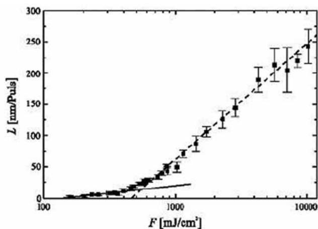
Figure 7.1: Ablation rates in Copper by S. Nolte [67].
