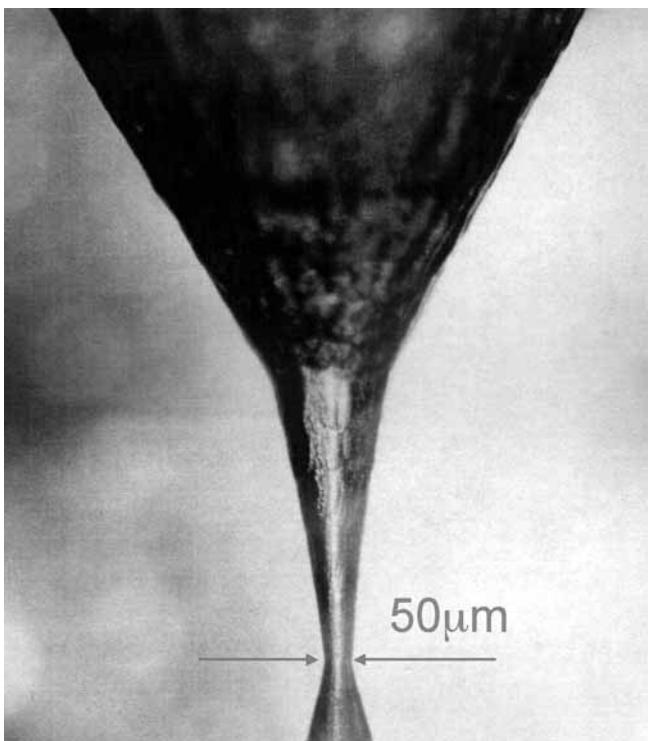
Figure 5.4 Diamond wire drawing die. Wire opening 50 $\mu\text{m}$ . Photo: Diamond Tools Group, Netherlands.
