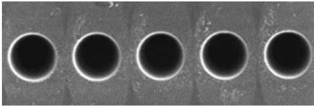
Figure 5.3. Array of ink jet nozzles drilled in 50  $\mu\text{m}$  thick polyimide.
