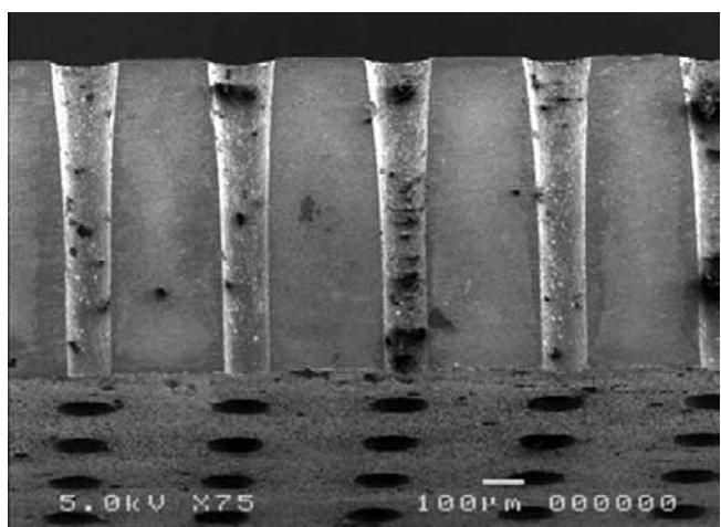
Figure 6.1. Array of 100 µm holes for medical filters.
