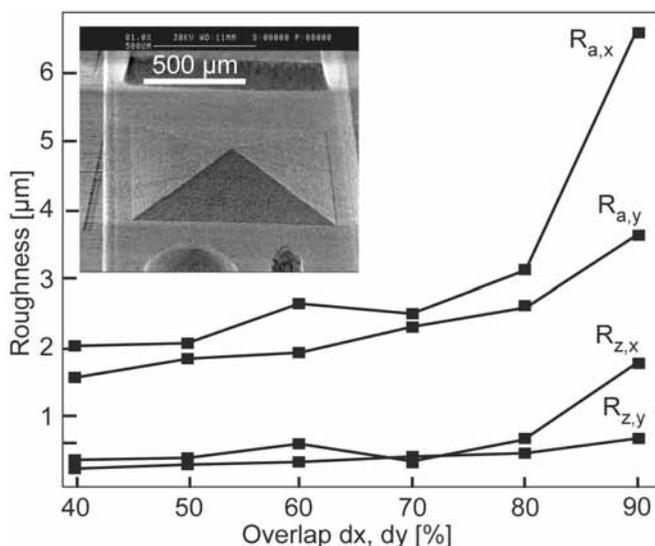
Figure 4.6: Surface roughnesses of WC after laser micro structuring ( $\lambda = 355\text{nm}$ ,  $f_p = 5\text{kHz}$ ,  $E_p = 0.26\text{mJ}$ ). Inlet: surface of WC-embossing tool ( $E_p = 0.3\text{mJ}$ ).
