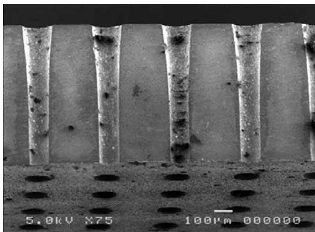
Figure 6.1. Array of 100 μm holes for medical filters.
