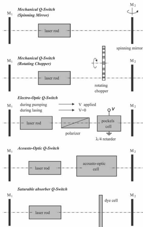
Figure 2.4. Different Q-Switching techniques
