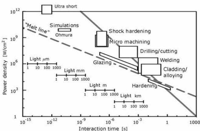
Figure 2.1: Overview of laser machining processes. The 'conventional' laser processes are found around the line of 1 kJ/cm<sup>2</sup>. The dotted line indicates the melt boundary of metal. Ultrashort processes require less energy per cm<sup>2</sup> in general.
