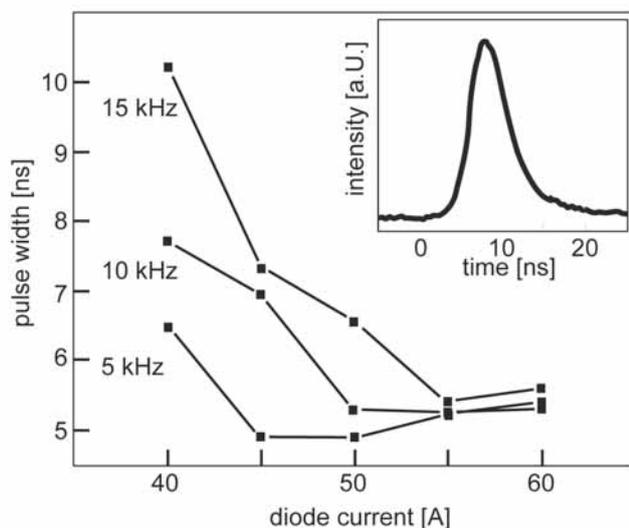
Figure 4.3: With the Innoslab concept shortest pulse durations of about 5 ns at 5 kHz repetition rate are demonstrated emitting a high quality nearly diffraction limited 5mJ laser pulse.
