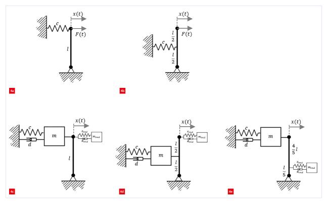
Analogy between design for high stiffness and optimal TMD placement.
