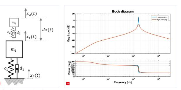
The effect of damping on machine dynamics. (a) Dynamic model with dx(t) as point of interest (POI), which is the relative displacement output between mass 1 and mass 2. (b) The Bode diagram shows the transmissibility from floor vibrations to this POI: dx(t)/x<sub>1</sub>(t). The difference in damping value is visible at the resonance frequency around 160 Hz.
