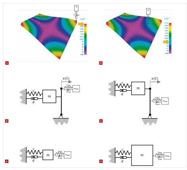
TMD placement on a structure. The upper figures (a and d) show the application of a TMD on a plate in two different positions. The middle figures (b and e) show the transmission ratio induced by the mode shape. The lower figures (c and f) show the representative dynamic model. Note the difference in effective mass in the lower two figures.
