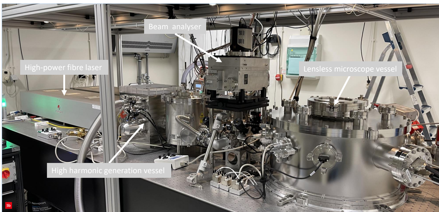
Overview of the table-top EUV SXR beamline with a lensless microscope as the end-station. The entire system fits on a 5-m optical table.
