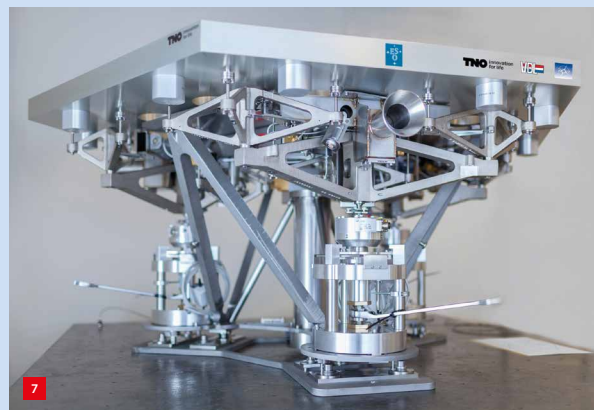
Prototype of M1 segment support (Image credits: TNO / Henri Werij)
