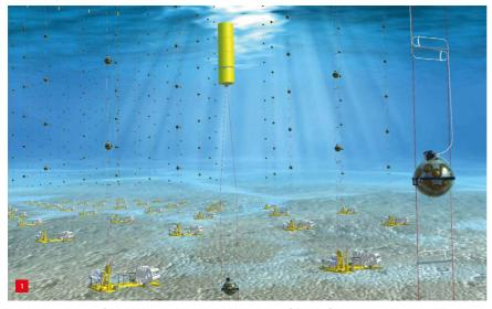
Artist's impression of the KM3NeT telescope at the bottom of the seafloor, comprising several thousands of spheres, equipped with photomultiplier tubes.
