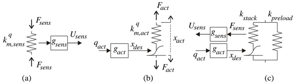
Figure 1 (a) Voltage-generating piezoelectric force sensor
