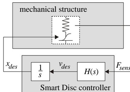
Figure 2 Illustration of energy dissipation based on Integral Force Feedback
