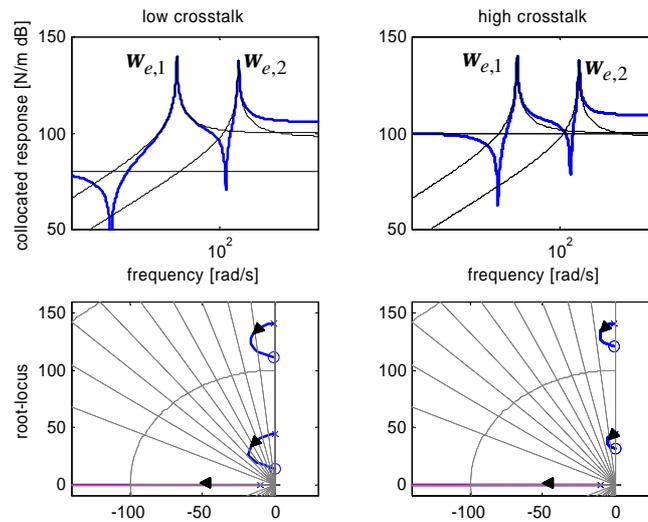
Figure 5 Illustration of the influence of crosstalk on the collocated frequency response and the IFF-root-locus
