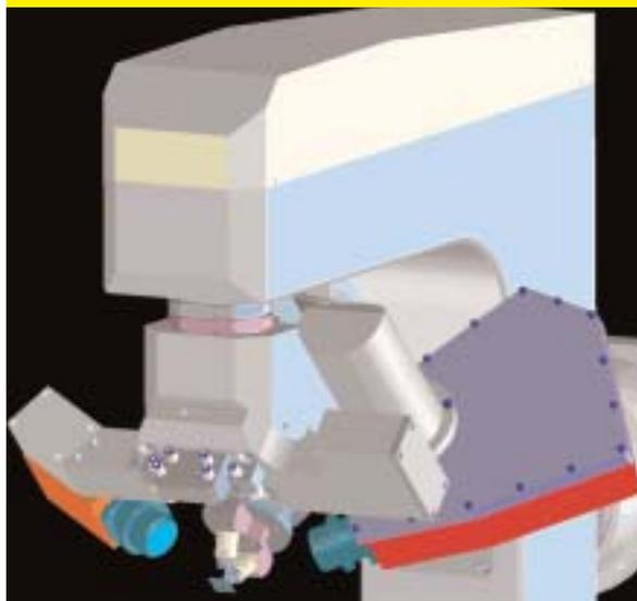
Detail of the Zeeko robot arm with nozzle and interferometer
