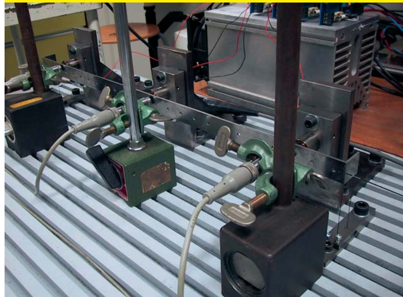
Flexible beam: an overactuated system with movement in one direction
