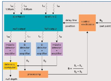
Controlling the null depth by using visible beams.
