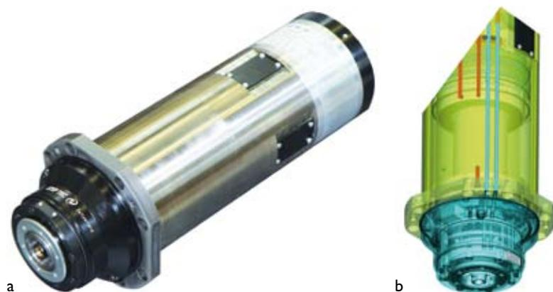
Figure 3. The StepTec tool spindle applied in Mikron HSM machines. (a) Overview. (b) Transparent view of the front nose showing the cooling channels.
