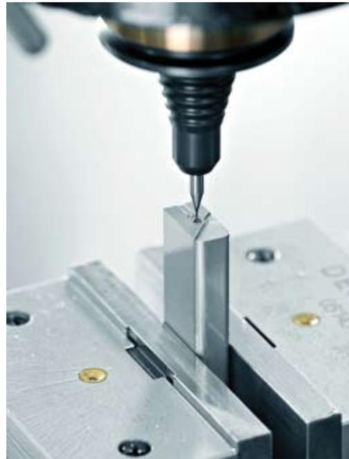
Figure 5. HSM milling a precision part.
