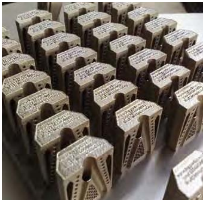
Figure 2. As design rules are packed in, SLM removes all obstacles in favour of extreme part optimisation.
