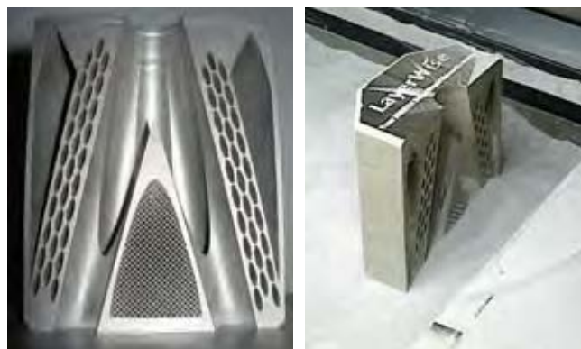
Figure 5. Usually, the products leaving the LayerWise facility can not be produced any other way. Shape complexity is not charged because the production cost is primarily dependent on the weight of the part.
