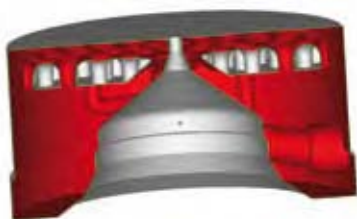
Figure 4. Injection moulding quality and speed can be increased by producing injection mould inserts with optimal cooling channels.
