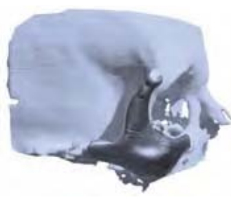
Figure 7. The complex shape of a zygoma implant was digitally derived through medical imaging and produced using SLM technology.
