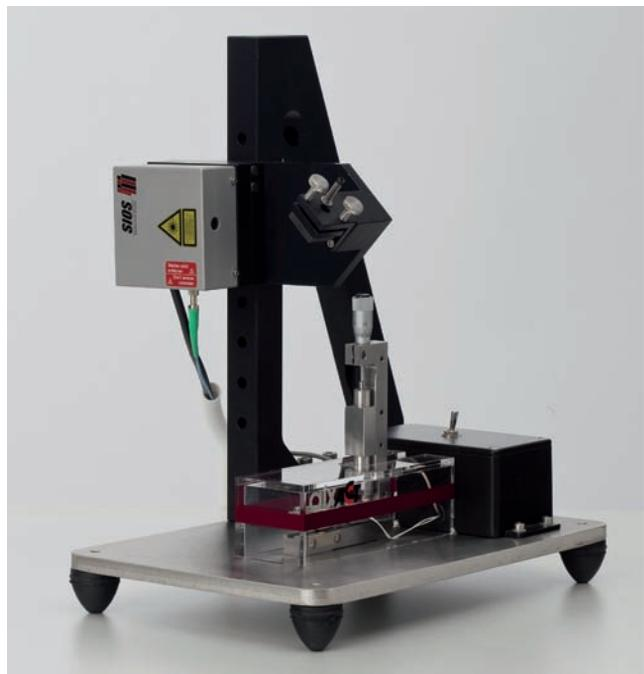
Figure 5. The aix4PB measurement system: four-point bending sample holder with connected single-beam laser interferometer.
