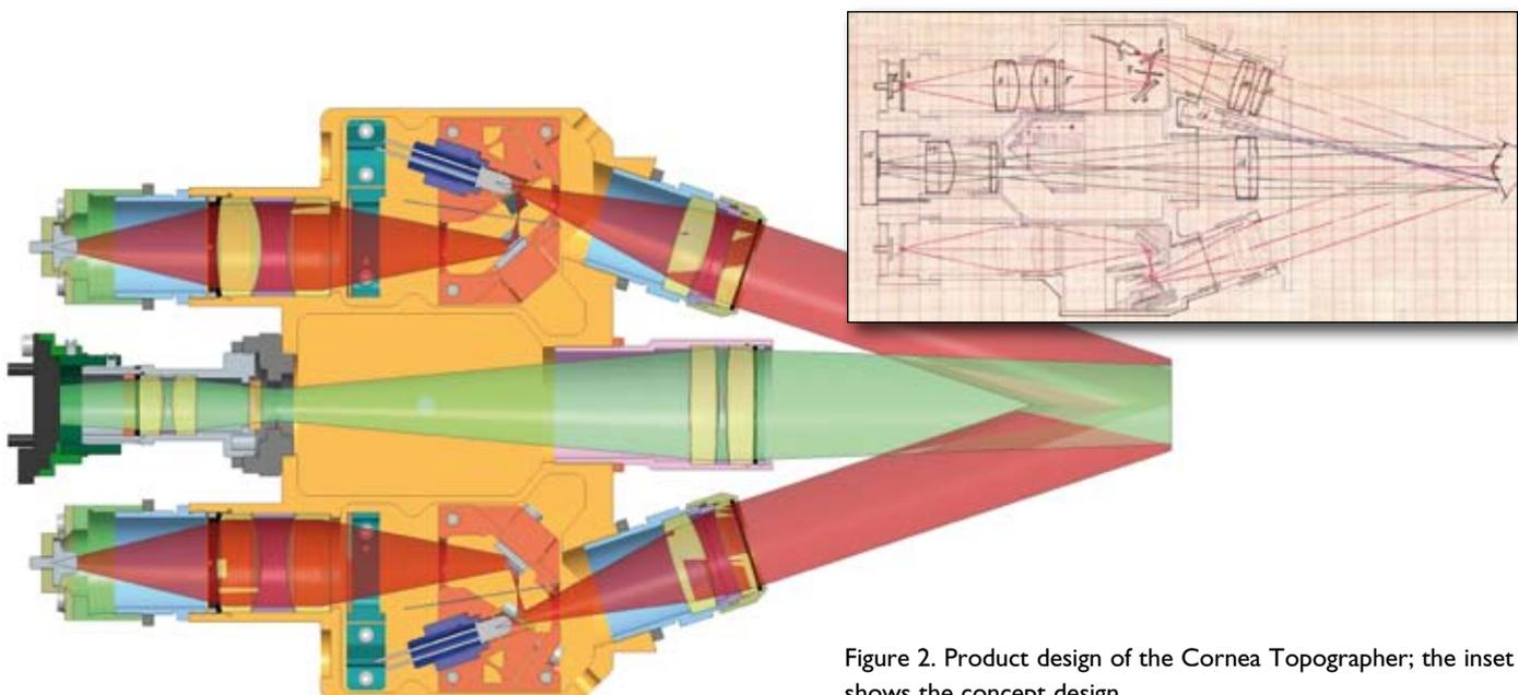
Figure 2. Product design of the Cornea Topographer; the inset shows the concept design.
