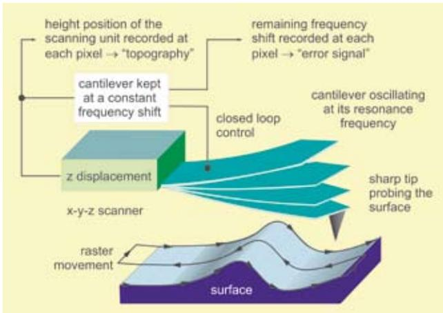
Figure 2. SFM working principle described for the dynamic mode with closed loop for constant force gradient imaging.
