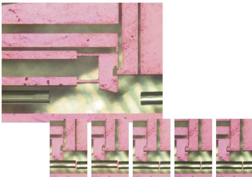
Figure 6. ID fiber positioning and clamping sequence, from (left) fabrication position, to (right) maintaining the fiber in position without using power.
