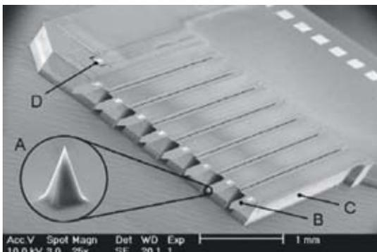
Figure 3. SFM chip of the MECA AFM [5].
