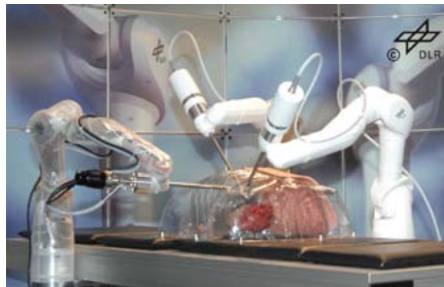
The DLR MiroSurge surgical robot. (Illustration: DLR)
