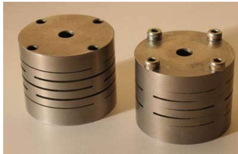
Figure 4. The harmonica bush, on the right in its 'locked state' with the four screws that are used for controlling the pretension.
