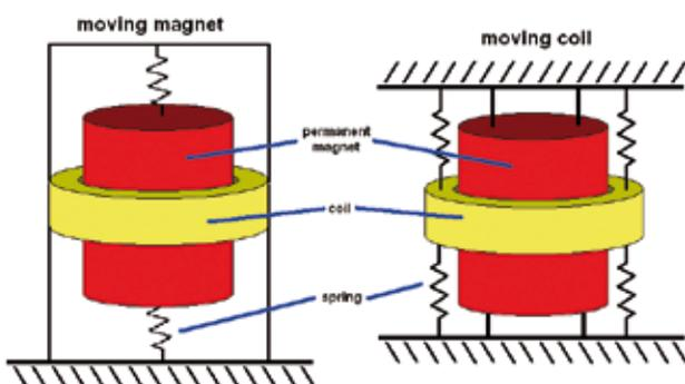
Figure 3. Geophone topologies: moving magnet (left) and moving coil.
