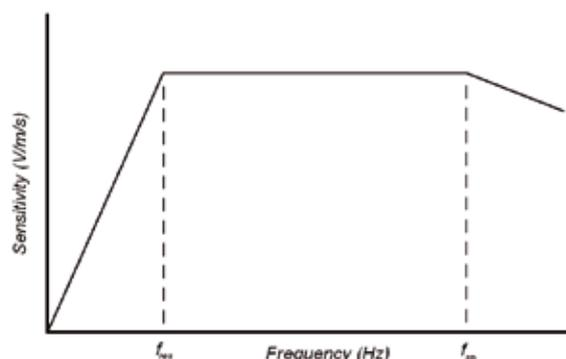
Figure 4. Response curve of a geophone.
