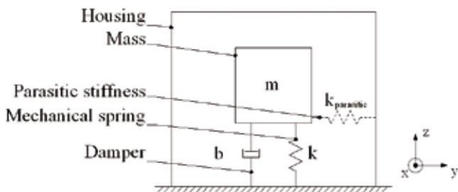
Figure 2. Mechanical geophone representation.
