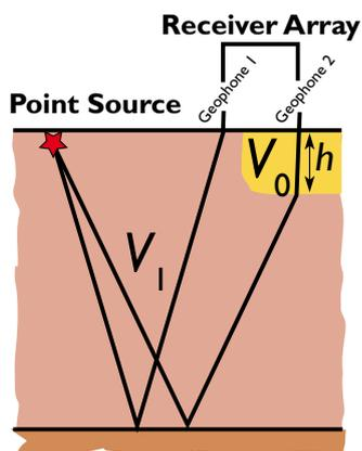
Figure 1. The principle of seismic measurement.
