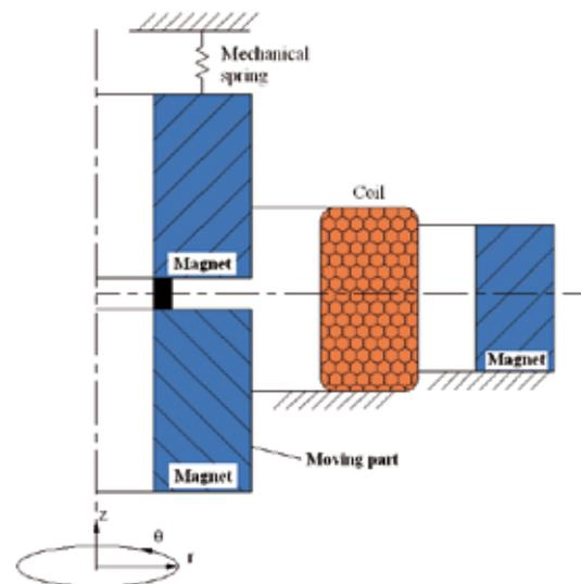
Figure 6. Geophone with passive magnetic spring.
