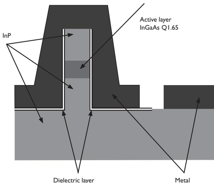
Figure 2. Structure of the metal-coated semiconductor nano-cavity laser.
