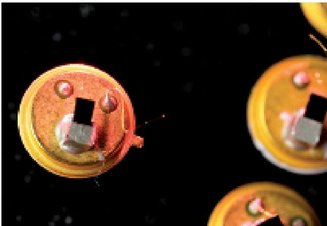
Figure 6. Some of Hill's metal-coated nano-cavity lasers. (Photo: Bart van Overbeeke)
