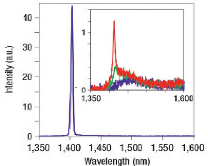
Figure 7. Measured light spectrum of the laser with a sharp peak at the 1400 nm wavelength. Inset: spectra just below and above the threshold current of 6  $\mu\text{A}$ .
