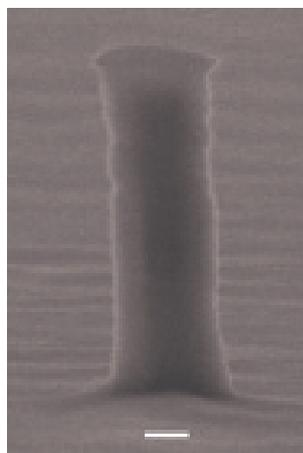
Figure 3. SEM image of the pillar-like laser structure.
