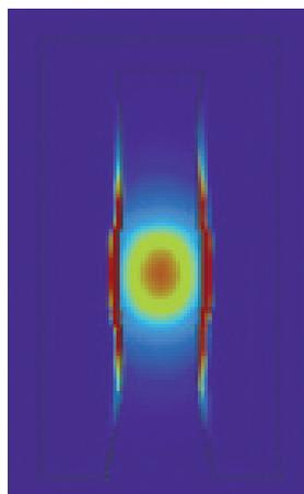
Figure 4. Simulated light distribution of the lasing mode.
