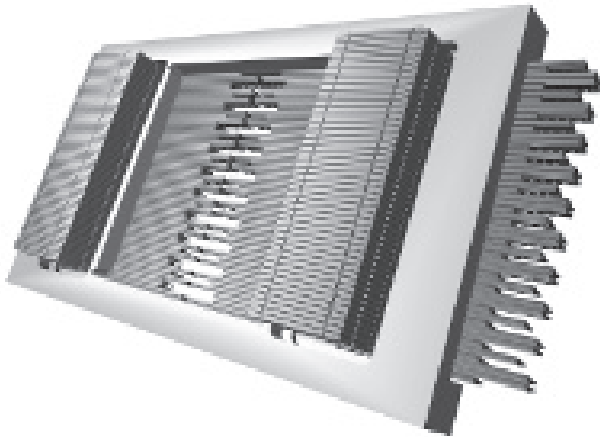
Figure 12. Design of a Configurable Slit Unit.
