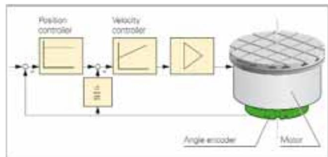
Figure 1. Control loop with rotational direct drive (torque motor).
