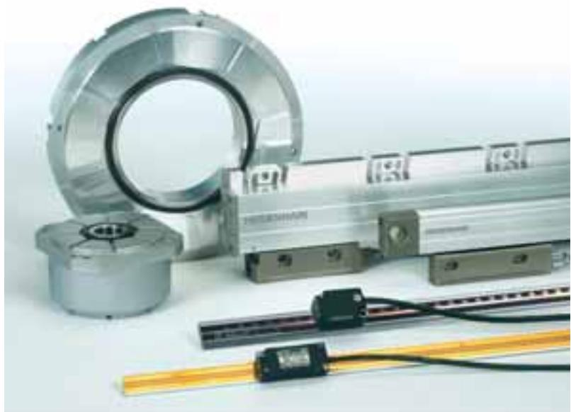
Figure 6. A selection of linear and angular position encoders for direct drives. Signal periods are as low as 4 µm or 36.000 per revolution. Maximum interpolation errors are as low as ± 0.04 µm or ± 0.4".
