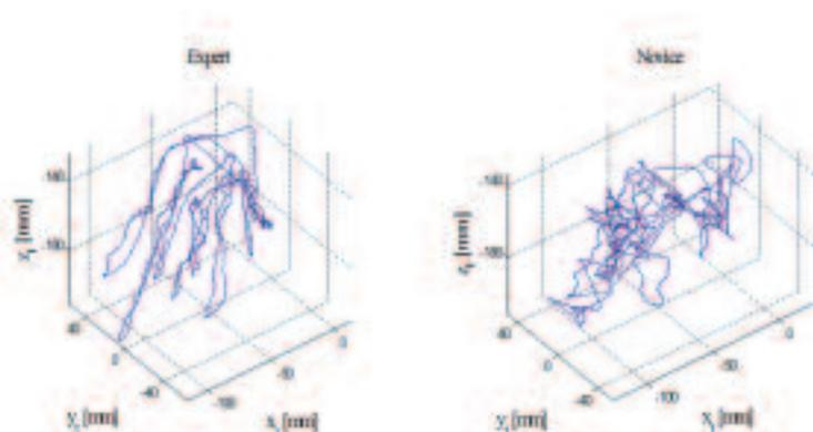
Figure 4. Typical instrument trajectories of an expert (left) and a novice (right) performing the positioning task. This figure shows that the motions of the expert separate eight points more distinctly than the motions of the novice.
