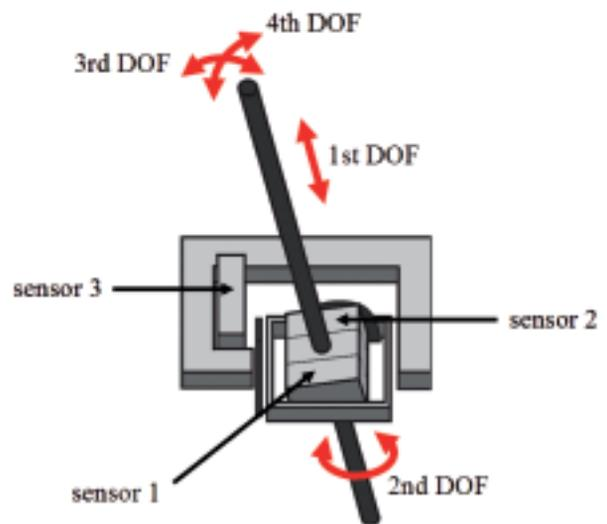
Figure 2. A schematic drawing of the TrEndo tracking system. The two-axis gimbal mechanism allows manipulation of the MIS instrument in four degrees of freedom. Sensor 1 measures the translation (1st DOF) and rotation (2nd DOF) of the MIS instrument around its axis. Sensor 2 measures left-right (3rd DOF) rotation of the instrument around the incision point. Sensor 3 measures forward-backward (4th DOF) rotation of the instrument around the incision point.
