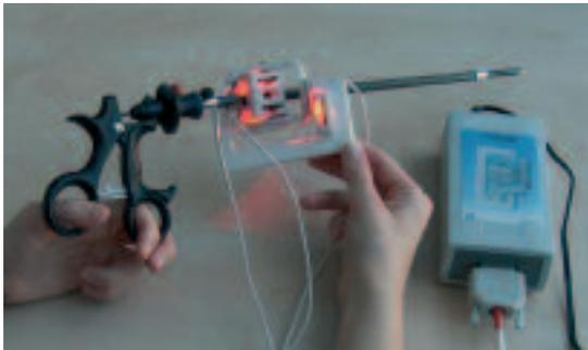
Figure 1. The TrEndo tracking system for guiding and measuring real MIS instruments in training setups.
