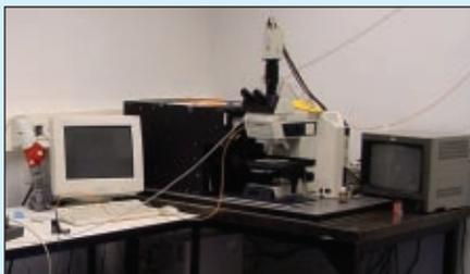
**Figure 1.** Raman microscope consisting of microscope with camera, spectrometer, computer and camera monitor
