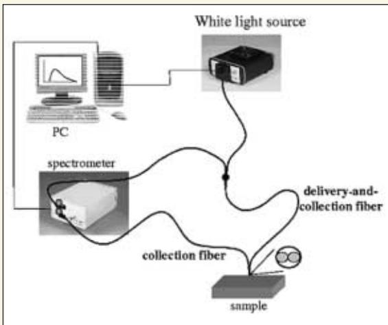
**Figure 3.** Schematic diagram of the DPS-setup.
