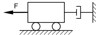
Figure 3: Simple model of linear SAW motor
