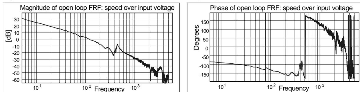
Figure 5: Open loop FRF of the linear SAW actuator.
