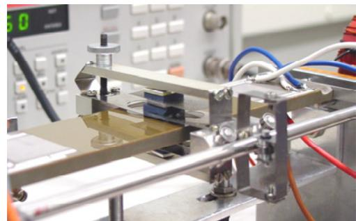
Figure 1 a) and b): Linear SAW motor with two sliders, preloading each other.
