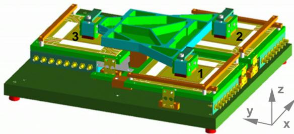
Figure 6: Design Planar SAW motor
