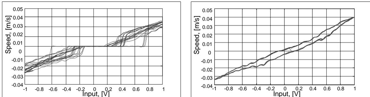
Figure 4: Measured open loop speed against input, a) dead band present, b) dead band solved.
