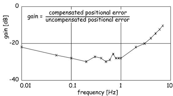
Figure 8. Frequency response of the active damping.
