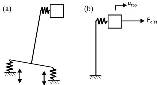
Figure 3. Approximate model of a non-rigid frame, the deformation of which is caused by
