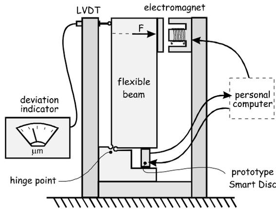
Figure 5. Schematic view of the experimental set-up.
