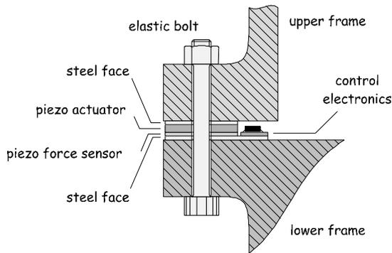
Figure 2. Envisioned realisation of the Smart Disc.
