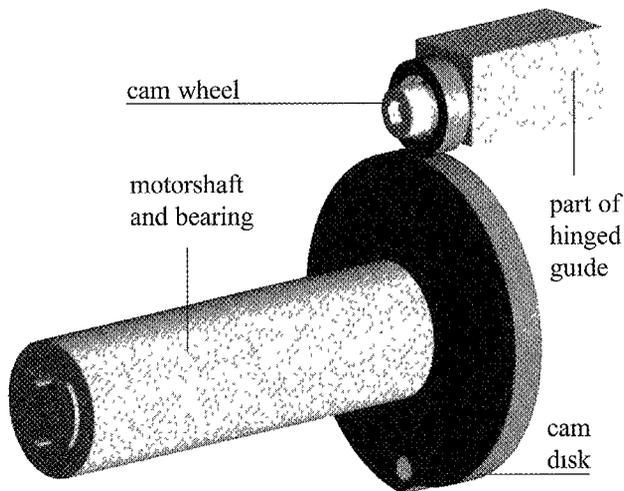
Figure 1 Transmission of drive system
