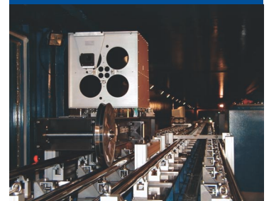
Cats Eye: part of delay line for the VLTi (made by Dutch Space and TNO TPD).
