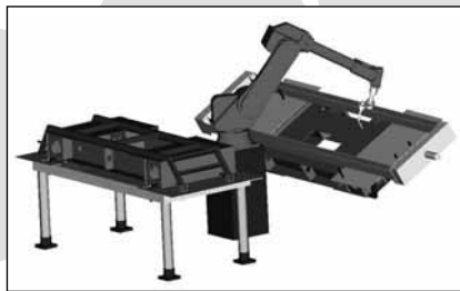
Lasrobot simulatie ACM pick & place frame Assembléon
