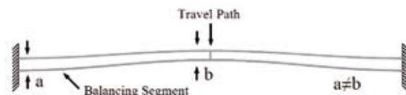
Figure 4. Concept of the statically-balanced compliant micromechanism of case II.
