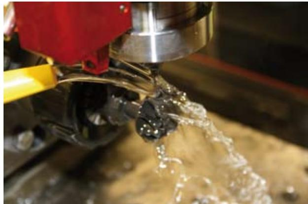
Figure 2. Micro-EDM milling of a turbine impeller ( $\varnothing 20 \text{ mm}$ ) made from  $\text{Si}_3\text{N}_4\text{-TiN}$ . (Photo courtesy K.U.Leuven)
