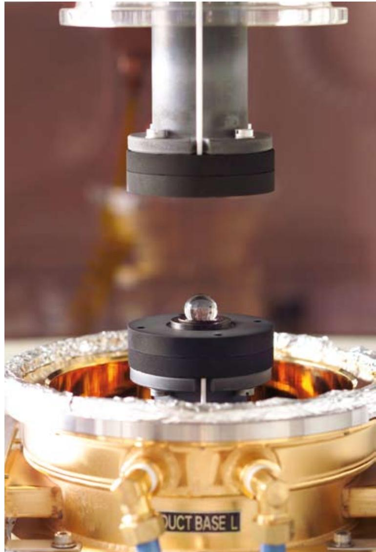
Figure 7. The Precision4 $\mu$  process for glass moulding.
