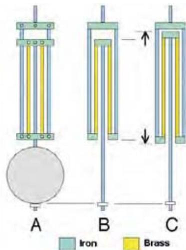
Figure 2. Harrison's gridiron pendulum clock. (Source: Wikipedia)
