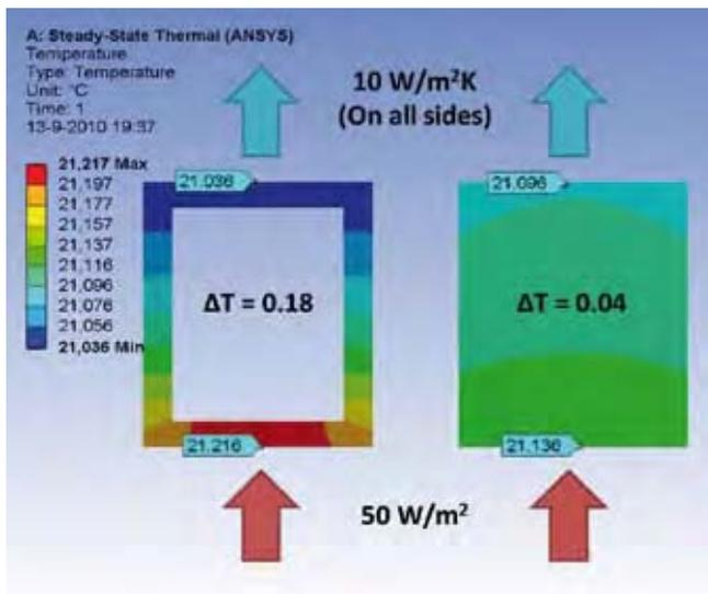
Figure 4. Cross sections: gradient reduction ~ factor 4.
