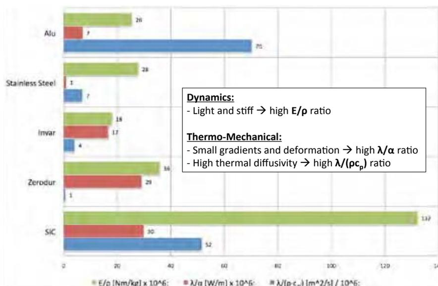
Figure 3. Material properties of some typical construction materials.
