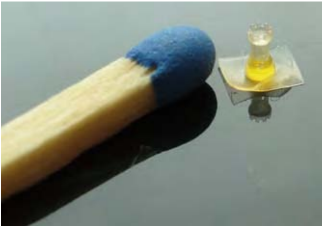
Figure 8. Miniature chess castle (height 2.8 mm) containing an internal staircase.
