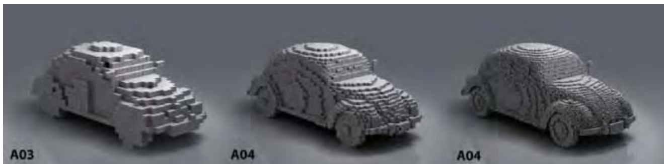
Figure 4. Principle of building a product with volumetric pixels (voxels) in different resolutions.
