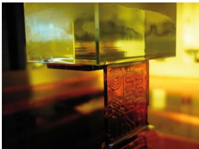
Figure 2. Building process of a microfluidic chip with internal canals.
