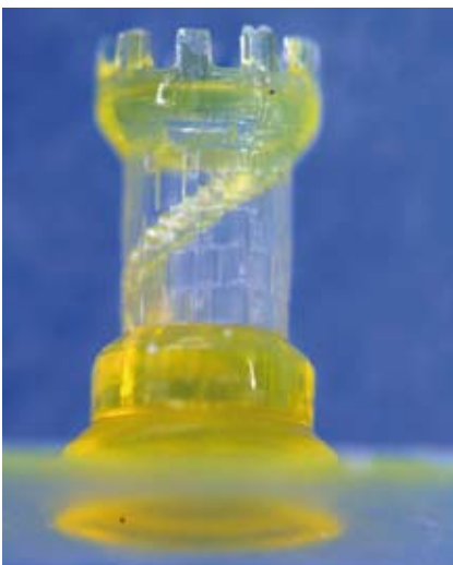
Figure 8. Miniature chess castle (height 2.8 mm) containing an internal staircase.
