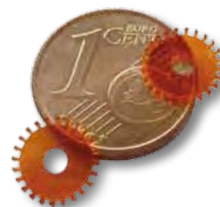
Figure 3. Miniature parts produced with microstereolithography.
