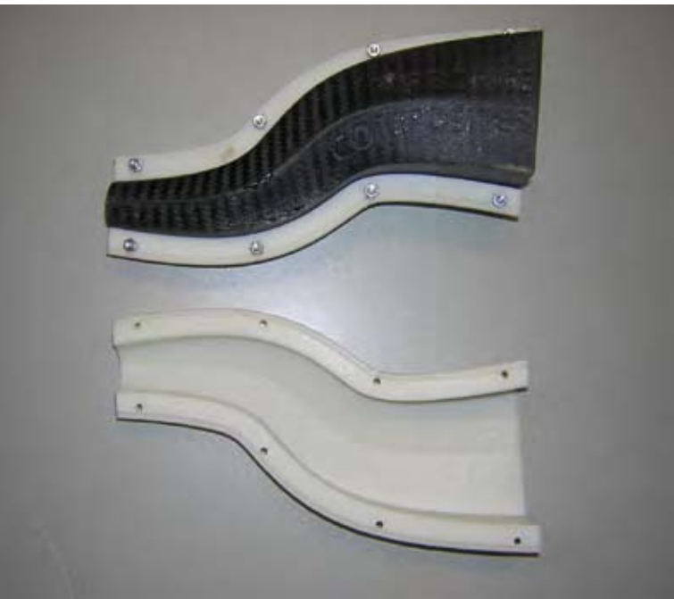
Figure 8. The polycarbonate mould produced with RM, for manufacturing complex-shaped composite products.
