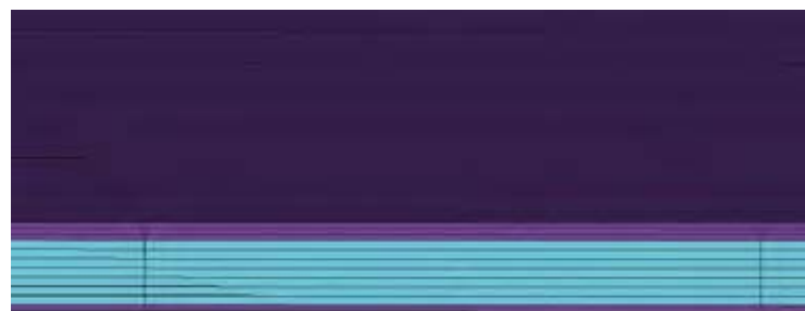
Figure 5. Different layers (the \pm 45^\circ fibres in purple, UD fibres in blue) in shell elements.
