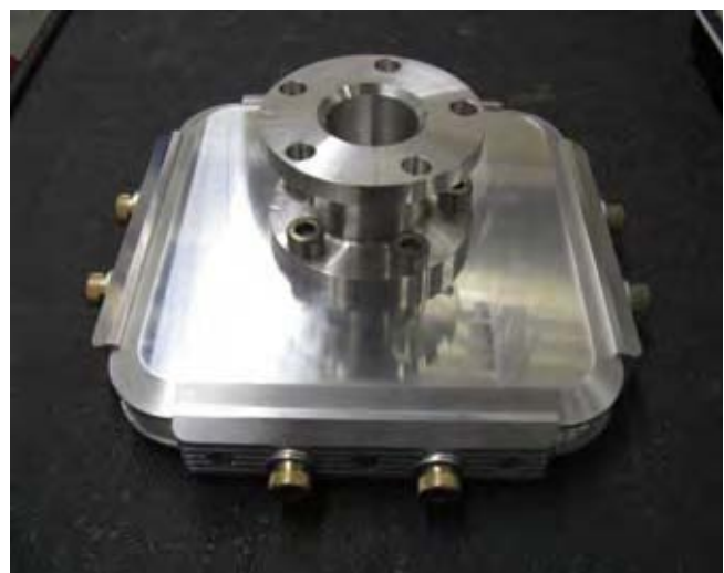
Figure 6. One of the metal prototypes of the vacuum chucks used in the test system.
