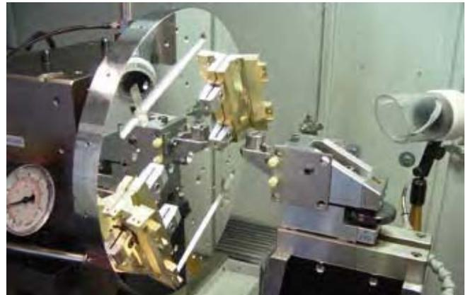
Figure 4. Diamond turning of a cylindrical mirror, which is a freeform surface, using the machine's slow tool servo.
