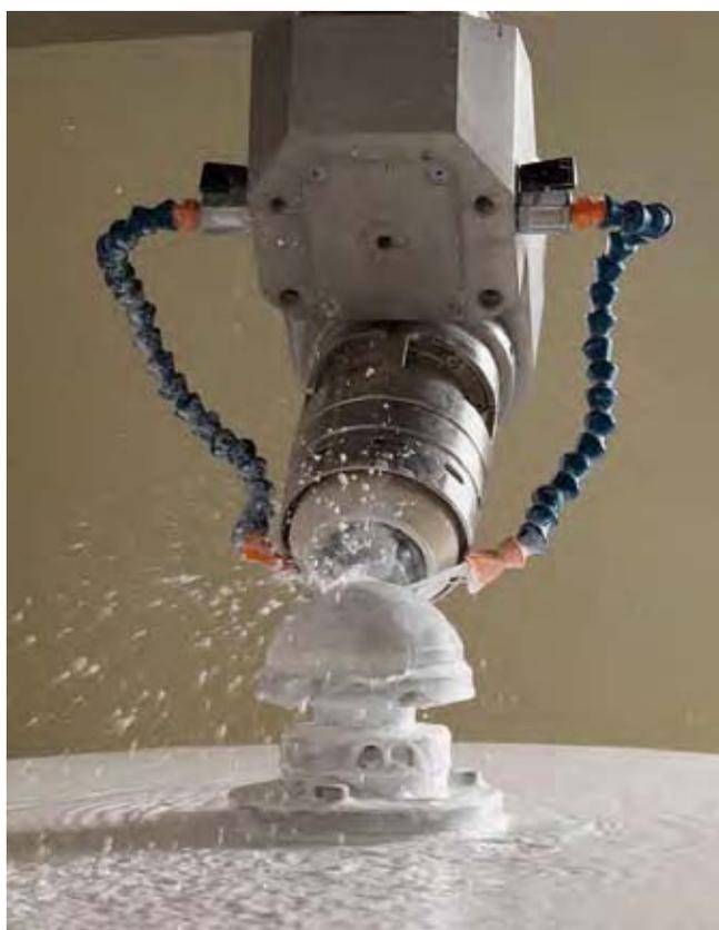
Figure 5. An aspherical surface on TNO's polishing robot.
