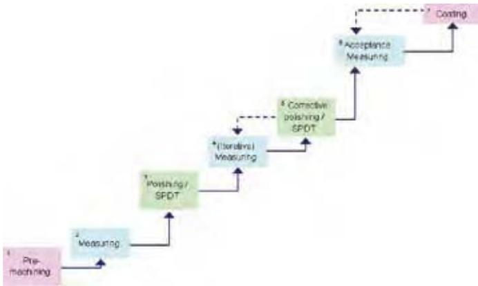
Figure 2. Value chain for freeform machining and metrology.
