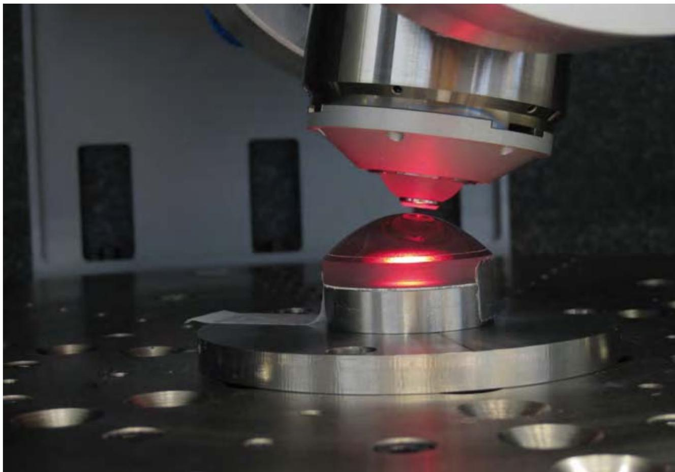
Figure 7. Measurement of a strongly curved convex asphere on NANOMEFOS.
