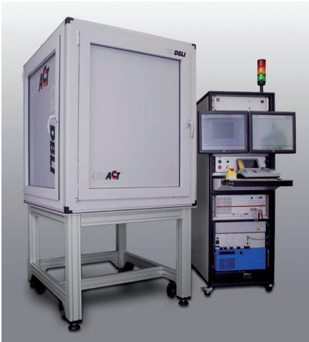
Figure 3. The aixDBLI system for automated wafer level measurements on wafer sizes up to 200 mm.
