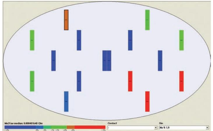
Figure 9. Wafer distribution of the transversal piezoelectric response of an AlN thin film deposited on a 150 mm wafer. Measured on bending structures cut from different positions on the wafer.
