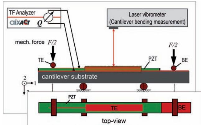
Figure 4. Measurement set-up to measure the transversal piezoelectric coefficient by the four-point bending configuration.
