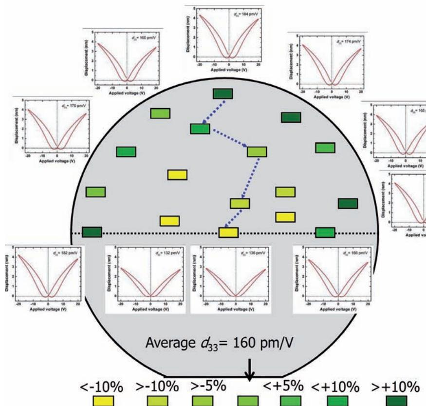
Figure 7. Wafer distribution of the large-signal displacement and derived average effective longitudinal piezo response of a PZT thin film (by courtesy of SolMateS).
