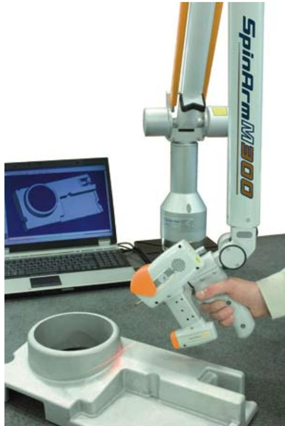
Figure 5. The SpinArm M 3D coordinate measuring machine for measurements based on laser scanning.
