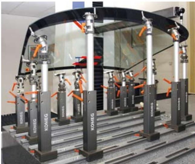
Figure 2. Clamping of a double-curved object with Koneg elements.
