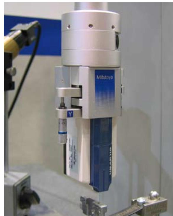
Figure 6. The UMAP-CMM swivelling microprobe may work with probe forces of only 1  $\mu\text{N}$ .
