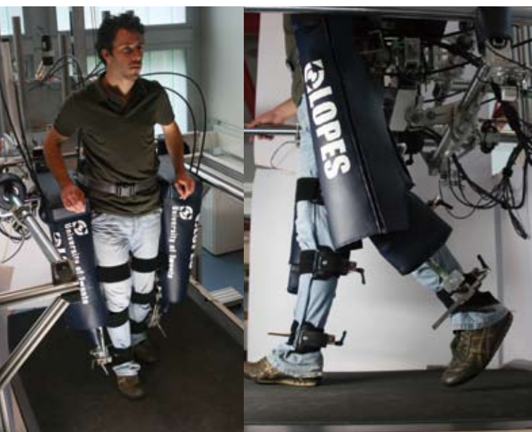
A test person using the gait rehabilitation robot LOPES. (Photos: RRD)
