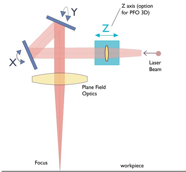
Figure 6. In a remote laser machining system two rotatable deflection mirrors allow the laser focus point to scan the workpiece.
