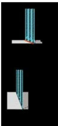
Figure 5. Cutting sheet metal with a small thickness gives a smaller incident angle than when cutting sheets with a larger thickness.
