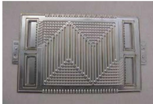
Figure 4. Example of precision welding a 200  $\mu\text{m}$  thick foil with a TruFiber 400 laser.
