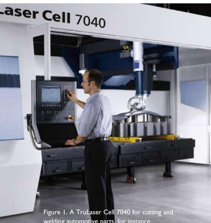
Figure 1. A TruLaser Cell 7040 for cutting and welding automotive parts, for instance.
