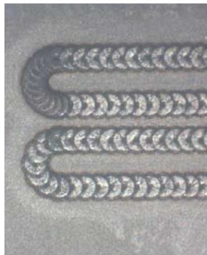
Figure 10. Frequency control of a TruPulse laser in curves. Upper track with fixed pulse frequency, lower track with fixed pulse overlap.
