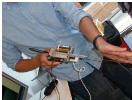
Figure 9. The lightweight robotic motion compensation instrument for mitral valve repair.
