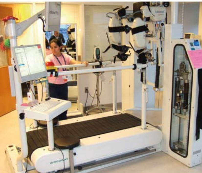
Figure 8. The Lokomat rehabilitation training robot in Spaulding's Motion Analysis Laboratory.
